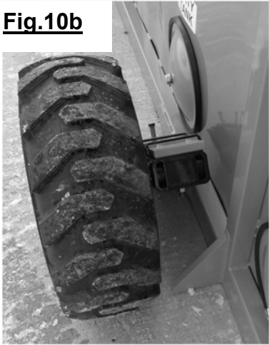
Rotating arm up. Sliding lock plate removed from under base frame gussett.
