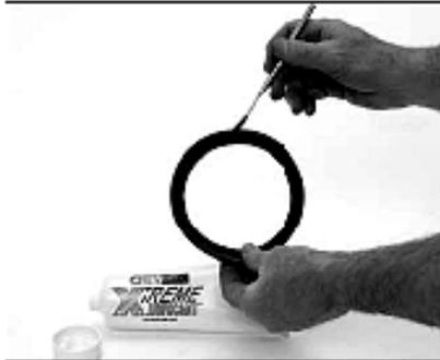
**1 CHECK & LUBRICATE GASKET**— Check gasket to be sure it's compatible for the intended service. Apply a thin coating of GUVLOK lubricant to outside and sealing lips of the gasket. Be careful that foreign particles do not adhere to lubricated surfaces.
