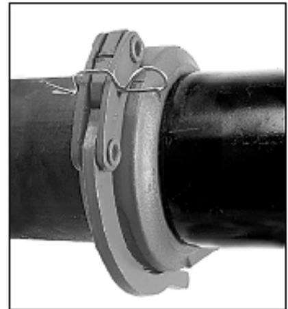
**6 ASSEMBLY IS COMPLETE**— Visually inspect the pipe joint to assure the coupling keys are fully engaged in the pipe grooves and the bolt pads are in firm even metal-to-metal contact on both sides of the coupling.
