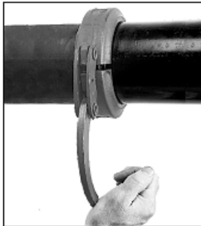
**5 LOCK COUPLING**— Fit the nose of the locking handle in the notch of the opposite housing. Press firmly down on the handle until it makes contact with the coupling housing. Insert locking pin into handle linkage to secure handle in closed position. (See Caution.)
