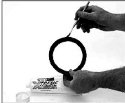
**1 CHECK & LUBRICATE GASKET**— Check gasket to be sure it is compatible for the intended service. Apply a thin coating of Gruvlok lubricant to outside and sealing lips of the gasket. Be careful that foreign particles do not adhere to lubricated surfaces.
