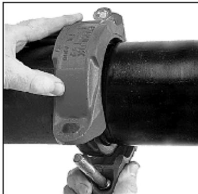
**4 HOUSINGS**— With one nut unthreaded to the end of the bolt, unthread the other nut completely and swing the coupling housing over the gasket, making sure the housing keys engage the grooves. Insert the bolt and turn the nuts finger tight.
