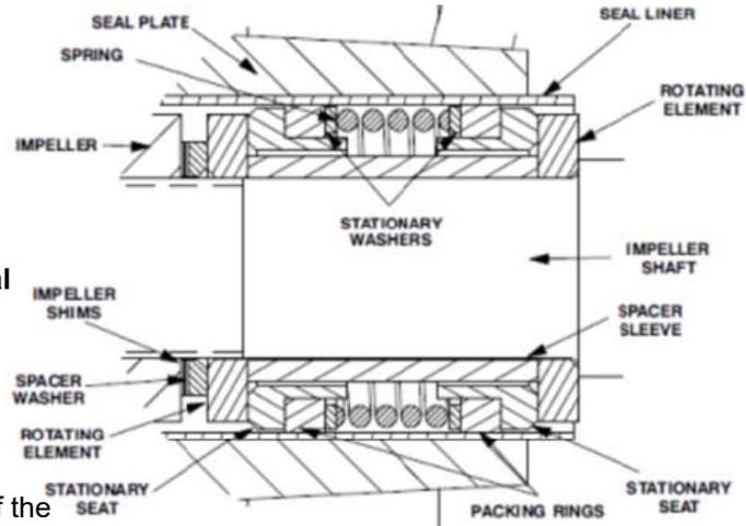
Installation of the inboard rotating element is dictated by the configuration of the shaft shoulder. If there is a radius at the shaft shoulder, the larger chamfer on the I.D. of the inboard rotating element must be positioned toward the shaft shoulder. If there is an undercut at the shaft shoulder, the larger chamfer must be positioned away from the shaft shoulder. Determine the correct position for the rotating element and slide it onto the shaft.
