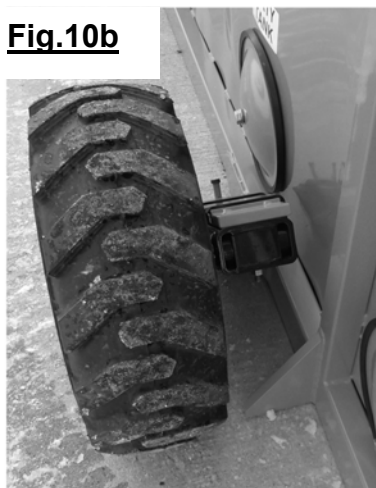
Rotating arm up. Sliding lock plate removed from under base frame gusset.
