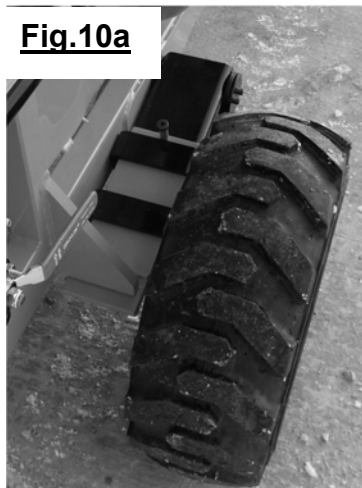
Rotating arm down. Sliding lock plate fully under base frame gusset.
