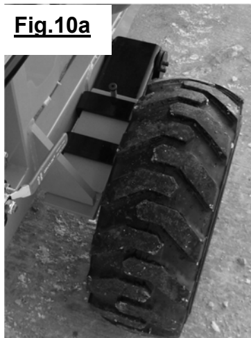
Rotating arm down. Sliding lock plate fully under base frame gussett.
