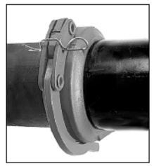
6 ASSEMBLY IS COMPLETE— visually inspect the pipe joint to assure the coupling keys are fully engaged in the pipe grooves and the bolt pads are in firm even metal-to-metal contact on both sides of the coupling.
