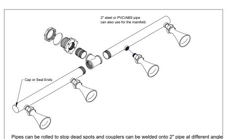
Typical horizontal installation in a tank
