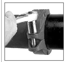
TIGHTEN NUTS— Tighten the nuts alternately and equally to the specified bolt torque. The housing bolt pads must make metalto-metal contact.
