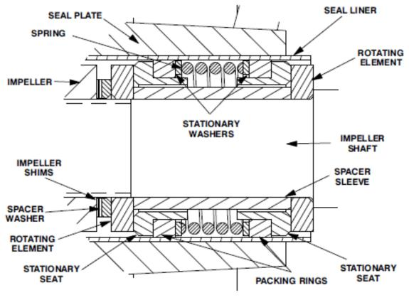
Figure 3. Seal Assembly
