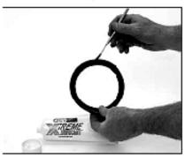
1 CHECK & LUBRICATE GASKET— Check gasket to be sure it is compatible for the intended service. Apply a thin coating of Gruvlok lubricant to outside and sealing lips of the gasket. Be careful that foreign particles do not adhere to lubricated surfaces.
