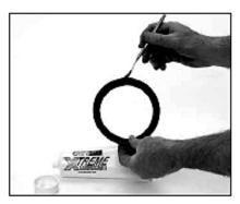
1 CHECK & LUBRICATE GASKET— Check gasket to be sure it is compatible for the intended service. Apply a thin coating of Graviok lubricant to outside and sealing lips of the gasket. Be careful that foreign particles do not adhere to lubricated surfaces.
