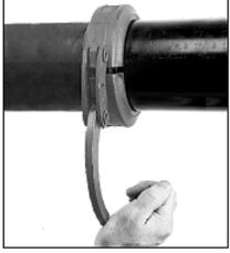
5 LOCK COUPLING— Fit the rose of the locking handle in the notch of the opposite housing. Press firmly down on the handle until it makes contact with the coupling housing. Insert locking pin into handle linkage to secure handle in closed position. (See Caution.)
