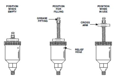
Figure 4. Automatic Lubricating Grease Cup
