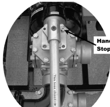
Valve Handles shown in the Cleaning/Treating Position
