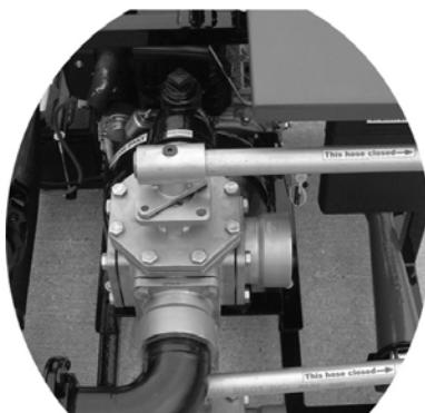
Valve Handles shown in the Mixing Position
