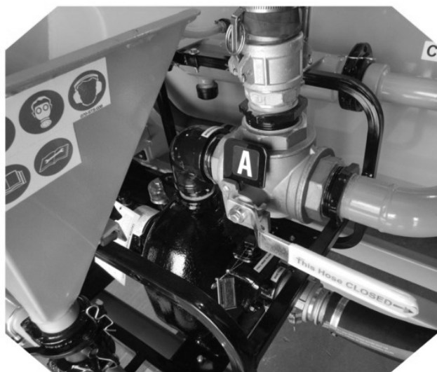
Valve Handle shown in the Processing/Transfer Position
