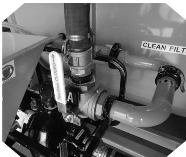
Valve Handle shown in the Mixing Position
