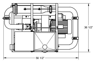
**Dimensions** Weight Hopper Height Mixing System Flow Valves Skid Frame Motor Pump
